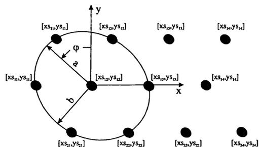
Fig.2: Deformed hexagonal points grid
