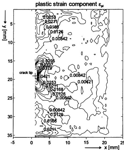
Fig.6.: Plastic strain component of equivalent strain.
