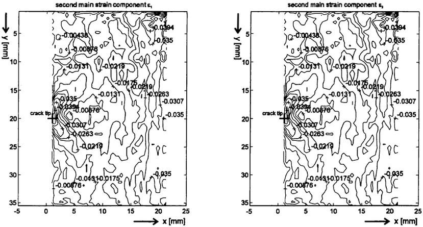
Fig 5: Main strains components
