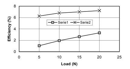
Fig. 4. Efficiency of the linear drive (Series 1) and toothed gear coupled with screw gear (Series 2)
