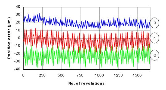
Fig. 2. Kinematic deviation of the screw position and hysteresis for drive unit B
