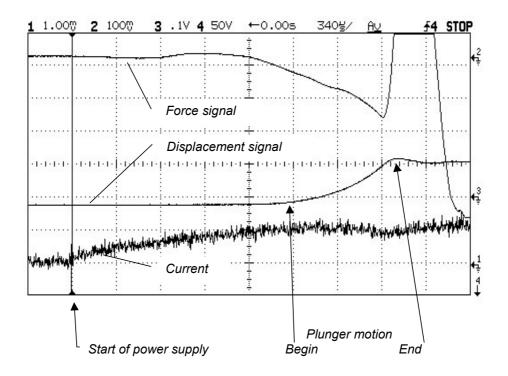
Fig. 6. Dynamic characteristics of small plunger electromagnet.
