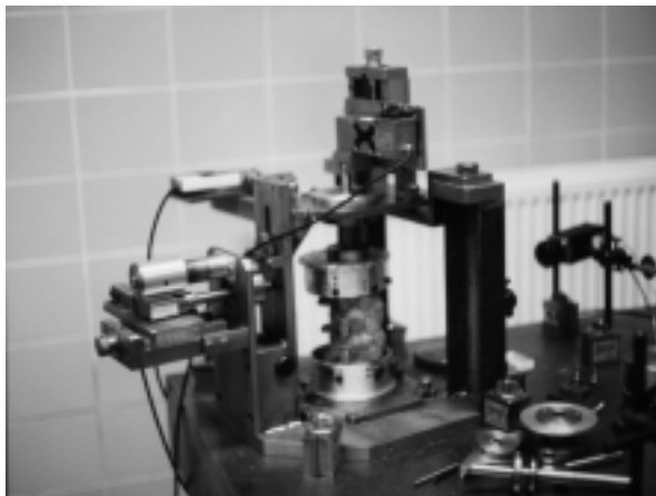
Fig. 1. The mechanical device that enables measurement of compression, torsion and bending of the sample
