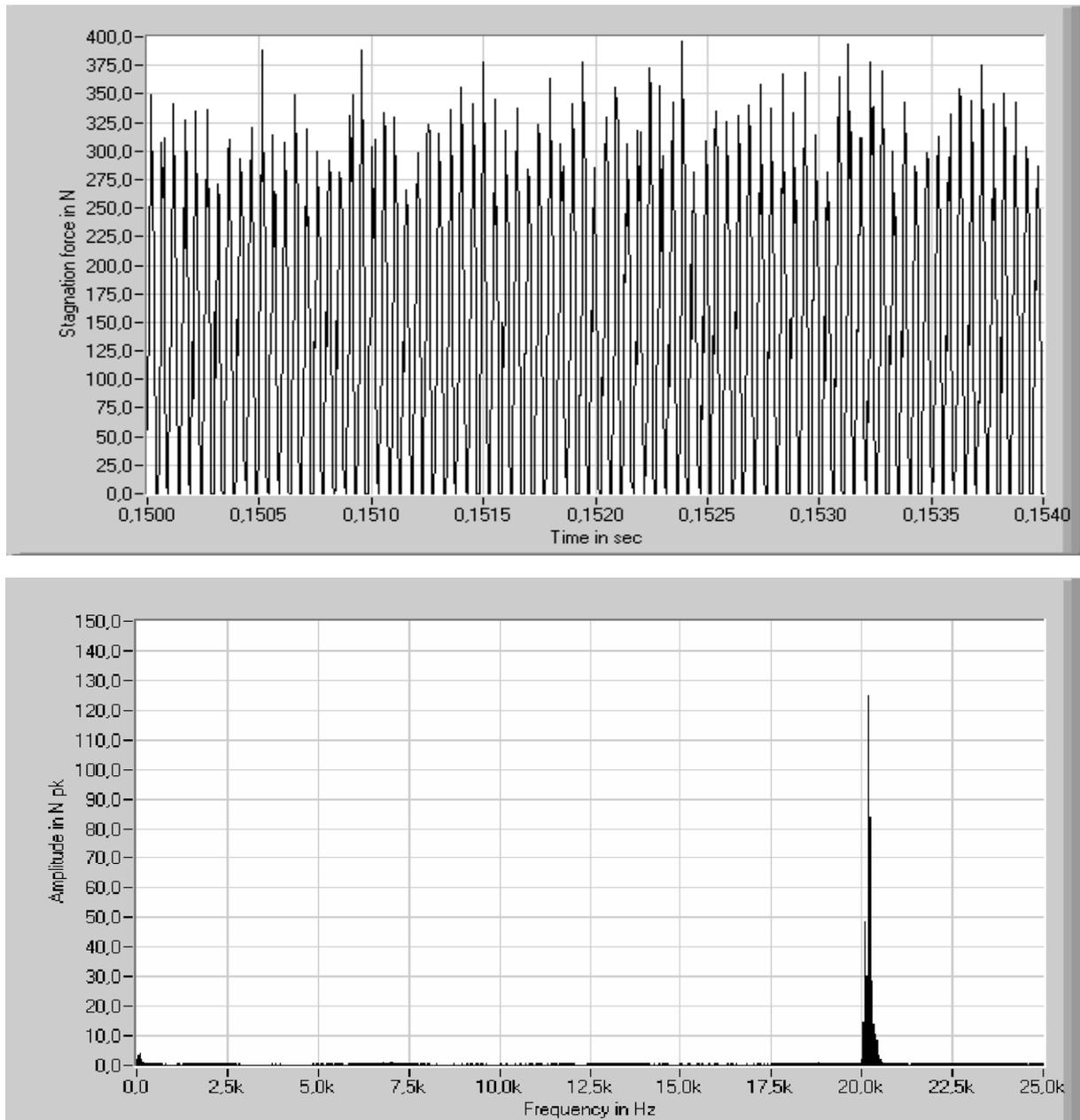
Fig. 3 Time and frequency domain of measured signal for modulated jet. (Testing conditions: operating pressure 20 MPa, nozzle diameter 1,98 mm, vibrating tip diameter 2,0 mm, tip position  $a$  12,2 mm, ultrasonic power 1 kW, standoff distance 40 mm.)
