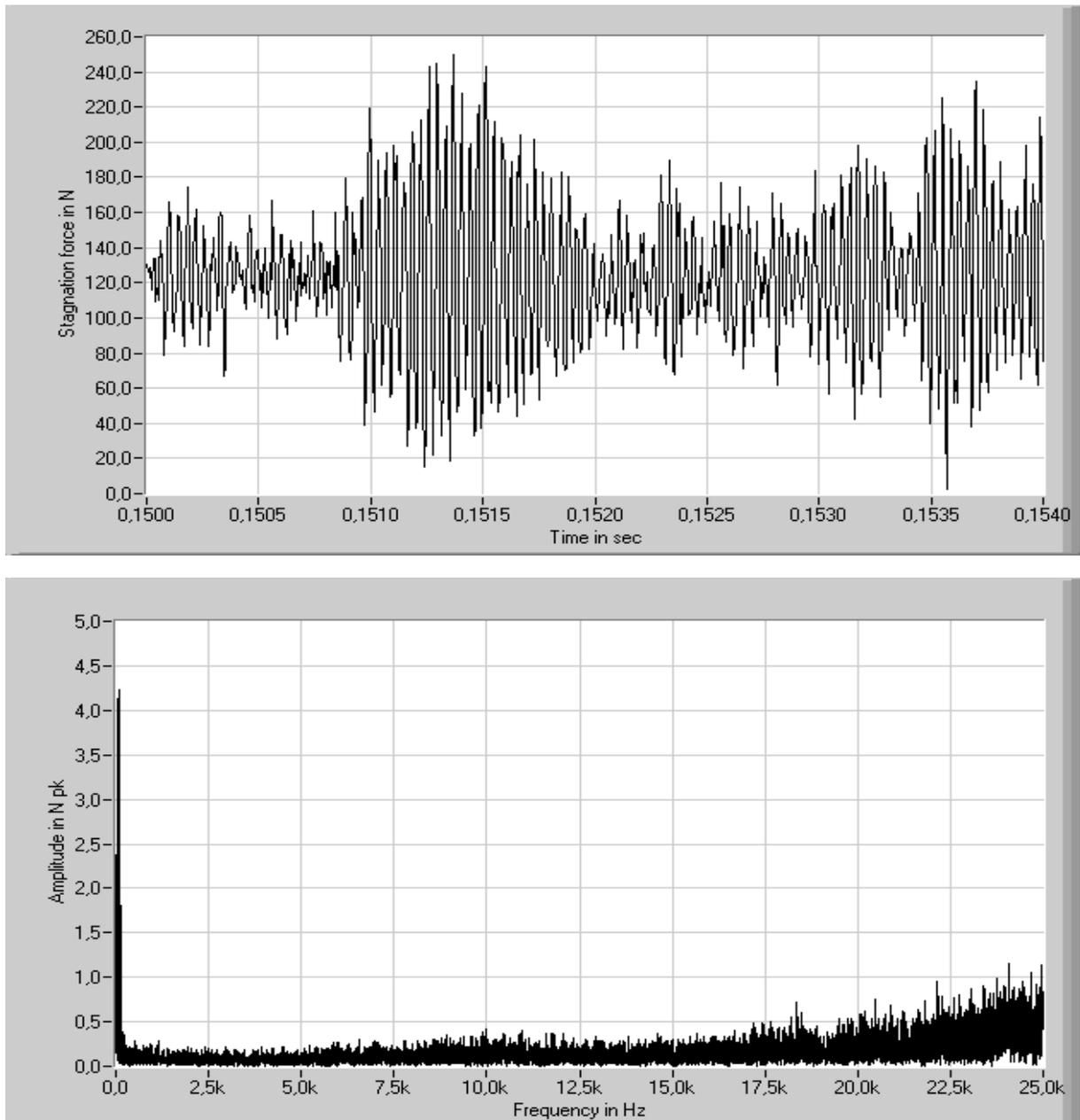
Fig. 4 Time and frequency domain of measured signal for continuous jet. (Testing conditions: operating pressure 20 MPa, nozzle diameter 1,98 mm, standoff distance 40 mm.)
