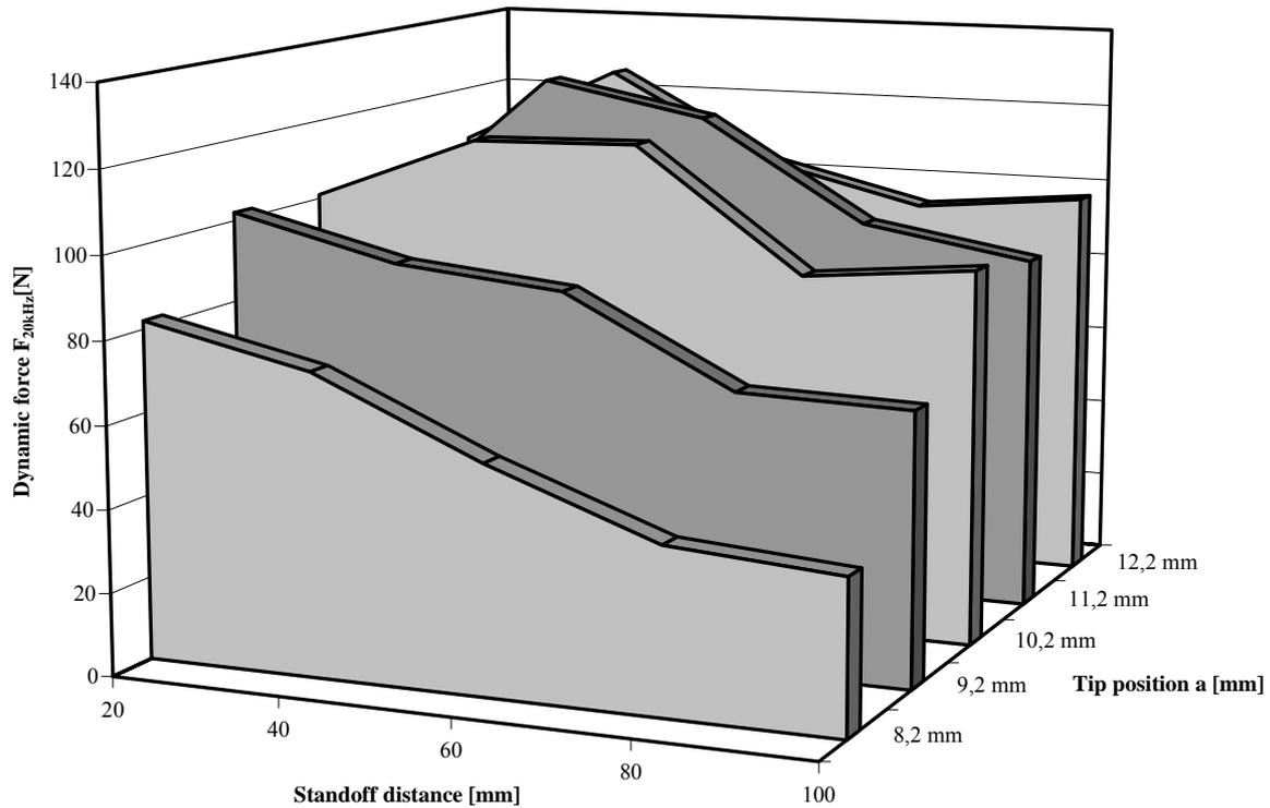
Fig. 5 Influence of the standoff distance and tip position on the peak amplitude of stagnation force (at 20 kHz). Testing conditions: operating pressure 20 MPa, nozzle diameter 1,98 mm, vibrating tip diameter 2,0 mm, ultrasonic power 1 kW.
