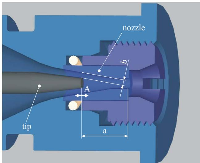
Fig. 1. Geometric configuration of the ultrasonic nozzle
