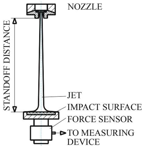
Fig. 2 Sketch of measurement of force effects of the jet
