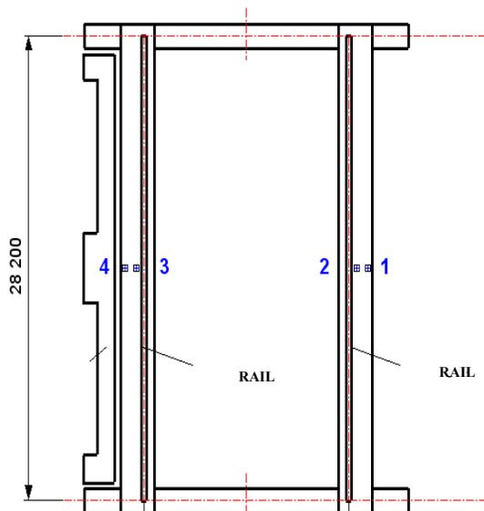
Fig.2 Scheme of the crane bridge and arrangement of tensometers
