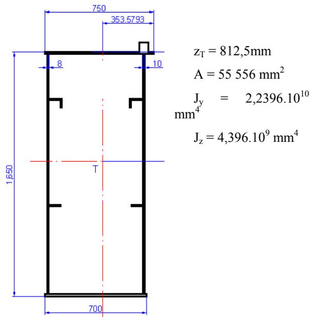
Fig.1 Cross-section of bridge crane beam
