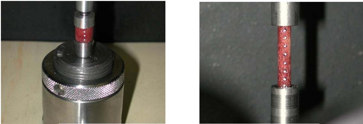
Fig.1 Compressive and tensile specimens with surface markers
