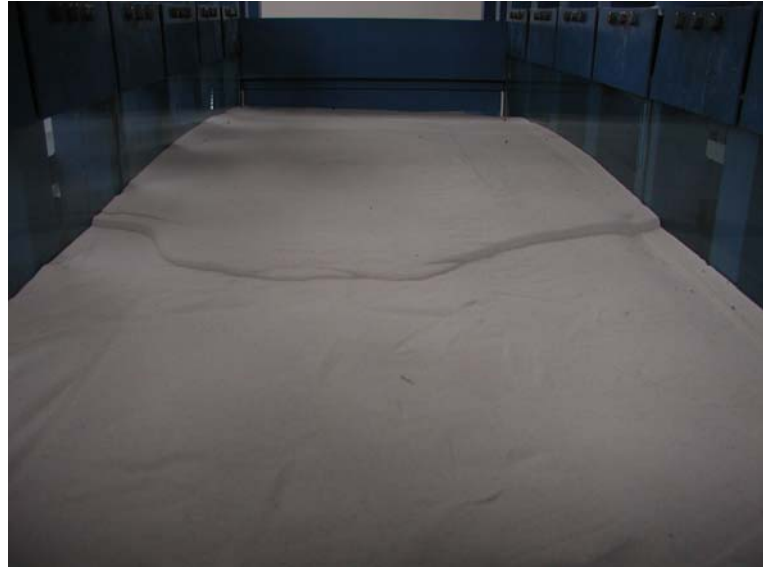
Figure 2 Deformed surface of the experimental mass from the back of the equipment after the toe movement of 134.8 mm on 18th Nov.2002 before the final movement of 159 mm. The top of moved front wall is above (blue).
