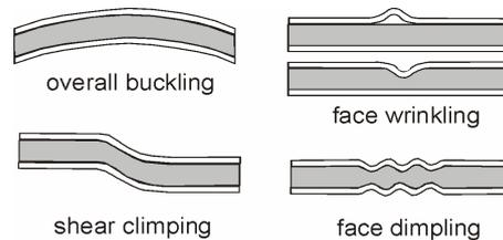
Fig.1 Instability modes for sandwich panels
