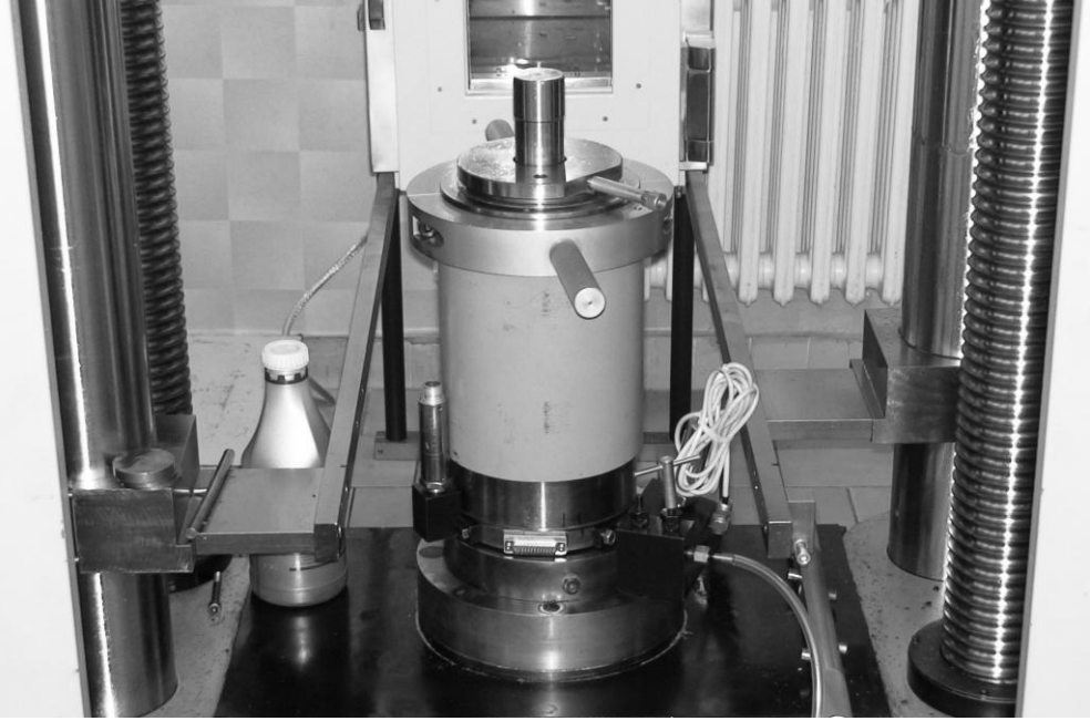
Fig. 1 Triaxial cell KTK 100 in mechanical press ZWICK 1494
