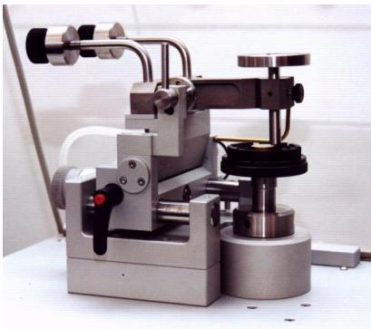
**Fig. 4** Tribometer ball-on-disc
