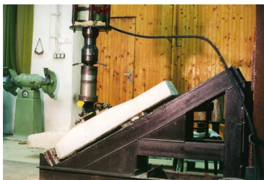
Fig. 6 Dynamic loading test
