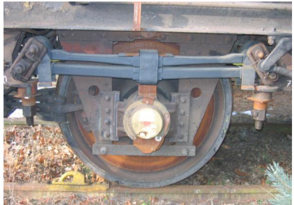
Fig. 2 The five-leaf parabolic steel spring and the two-leaf composite spring
