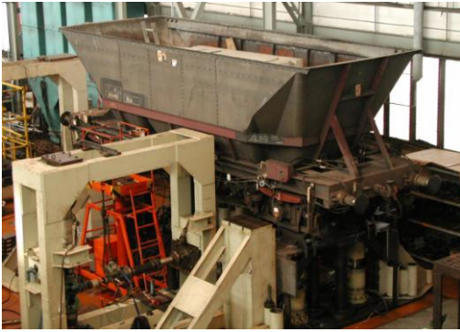
Fig. 1 The MGR Coal Hopper HAA wagon on the test stand in the Dynamic Testing Laboratory ŠKODA VÝZKUM s.r.o. – the real wagon and the multibody model visualization
