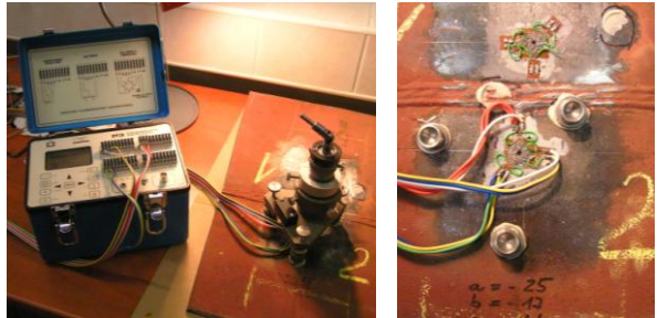
Fig. 4 Apparatus P-3 during drilling (left), hole in location 2 (right).
