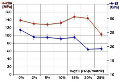
Fig. 2 Ultimate strength in bending *Rfm* and modulus of elasticity in bending *Ef* of composites with HAp nanopartricles
