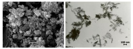
Fig. 1 SEM and TEM pictures of agglomerated needle-shaped nano HAp
