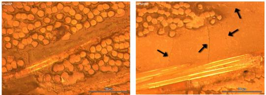
**Fig. 3** Pictures of polished cross-section of composite with 5% HAp (left) and 20% HAp (right) illustrate multiple cracking in cured matrix with higher amount of HAp
