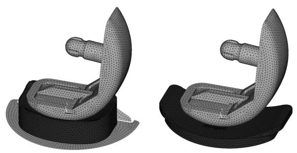
Figure 5: Meshed models of both unicondylar knee replacements types
