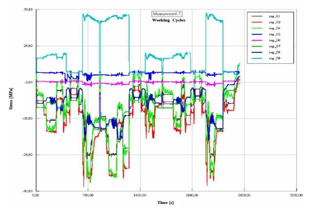
*Figure 9: Time behaviours of relative deformations converted to stress values for measured working cycle.*
