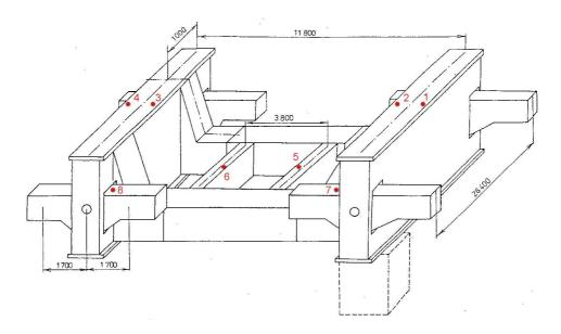
*Figure 1:* Scheme of the foundry crane 250t / 63t / 12, 5t - 26, 4 m with marked points of strain gauge arrangement
