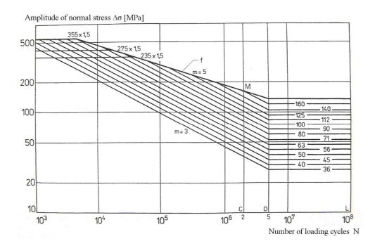
*Figure 10:* Dependence between amplitude of normal stress  $\Delta \sigma$  and number of loading cycles N for various categories of details
