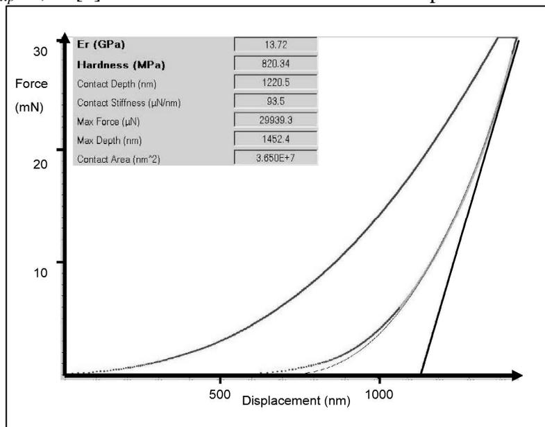
**Figure 3:** Load-displacement curve obtained during nanoindentation testing. The depth of the contact circle and slope of the elastic unloading allows specimen modulus and hardness to be calculated.
