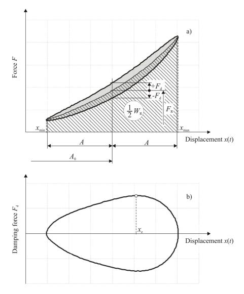
Figure 1: Measured force responce and its decomposition
