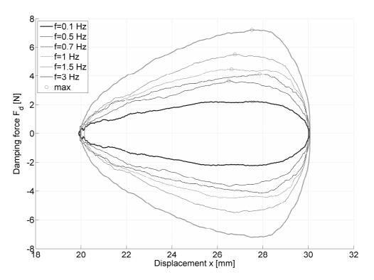
Figure 4: Damping force response
