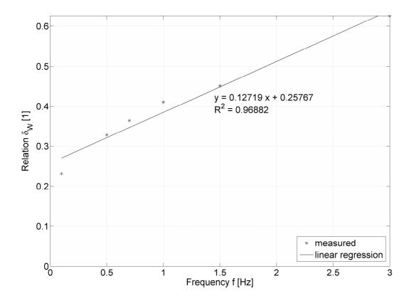
**Figure 6:** Dependence of relation  $\delta_W$  on exciting frequency f
