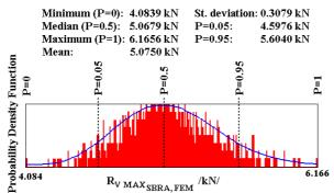
**Figure 11:** Maximum Total Reaction Forces in the Bit (SBRA-FEM Results of 500 Monte Carlo Simulations) and their Evaluation.
