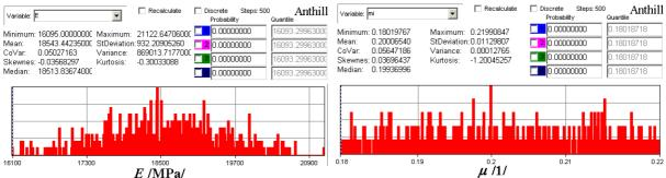
Figure 6: Stochastic Inputs for the Material of the Ore (Histograms of Young's Modulus and Poisson's Ratio).
