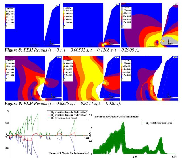
**Figure 10:** Reaction Forces in the Bit - SBRA-FEM Results (Results of one Monte Carlo Simulations and Results of 500 Monte Carlo simulations).
