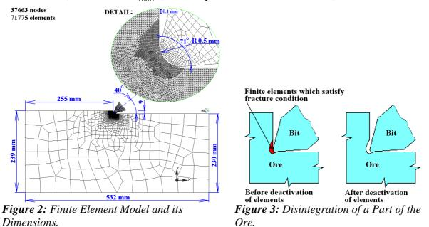
When the situation  $\sigma_{\rm HMH} \ge R_{\rm m}$  occurs (i.e. the equivalent stress is greater than the tensile strength) in some elements of the ore, then these elements break off (i.e. these elements are dead). Hence, a part of the ore disintegrates. In MSC.Marc/Mentat software, this is done by deactivating the elements that satisfy the condition  $\sigma_{\rm HMH} \ge R_{\rm m}$ . This deactivation of the elements was performed in every 5<sup>th</sup> step of the solution, see Figure 3.
