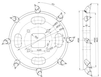
*Figure 13: Final Shape of Excavation Tool for Platinum Ore Disintegration Process.*
