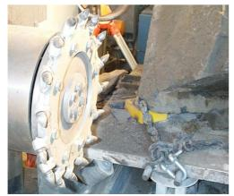
*Figure 1: Typical Example of Mechanical Interaction between Bits and Hard Rock (Ore Disintegration Process).*
