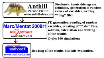
*Figure 7:* Computational Procedure - Application of the SBRA Method and FEM (Solution of the Ore Disintegration Process.
