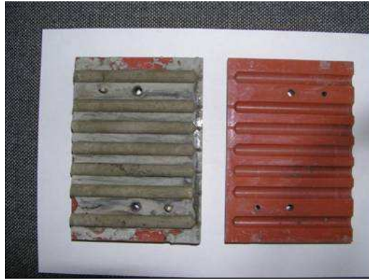
Figure 1: Plastic mould with specimen.
