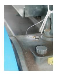
Measurements and frequency analyses were realized in the frequency range 2-800 Hz with rotations 600-1300 rpm (fan without loading), 1100 rpm during limited operation of fan (maximal allowable rotations with respect to crash of one fan) as well as with continual change of rotations 1100 to 1400 rpm during operation for one case allowed by operator.
