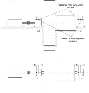
Figure 1: Scheme of supports positioning for fixation of sensors on bearing houses of fan.
