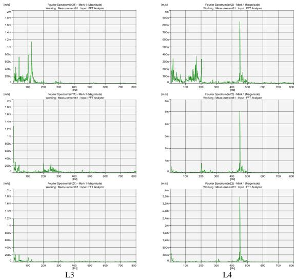
Figure 4: Frequence dependencies of velocity for 1100 rpm.
