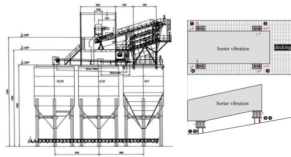
*Figure 5: Positioning of sorter on carrying structure.*
