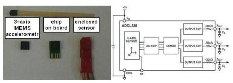
Fig. 2. Subminiature 3-axis accelerometer and its block diagram.
