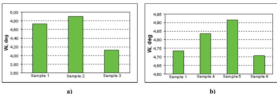
**Fig. 4.** Average values of the width of the {211} diffraction line obtained from areas P1 and P2 from the surface; a) relation of residual stresses on the feed modification, b) relation of residual stresses on the cutting speed modification.
