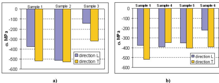
**Fig. 3.** Average values from areas P1 and P2 of residual stresses  $\sigma_L$  and  $\sigma_T$  from the surface; a) relation of residual stresses on the feed modification, b) relation of residual stresses on the cutting speed modification.
