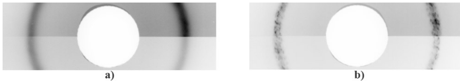
Fig. 2. Diffraction patterns of \alpha -Fe {211} lines obtained at the surface (a) of the ground sample A1N and after removal of 0.4 mm thick layer (b).
