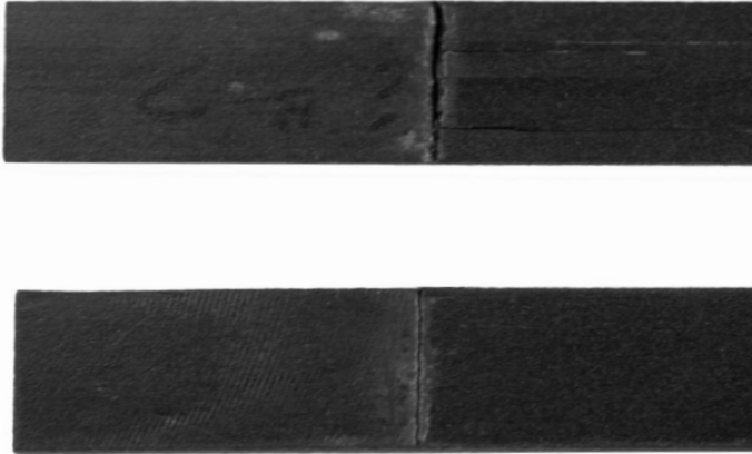
Fig. 7. Damaged composite specimens.
