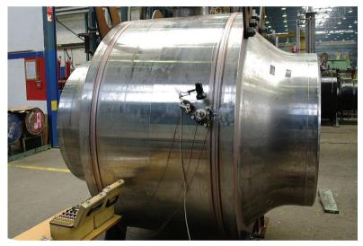
Fig. 1. Welded ball valve.
