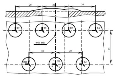
Fig. 4. Places of measurement around weld axis.
