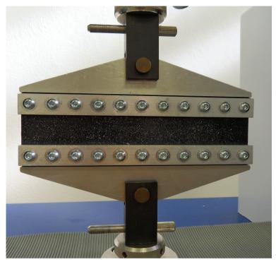
Fig. 1. Pure shear test device.
