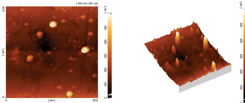
**Fig. 5.** Sample F as scanned with AFM (2D and 3D image) at 85 % r.h. in time K
