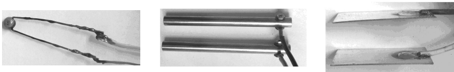
Fig. 4. Photos of measuring fixtures (from left to right): temperature sensor, resistance measuring bars and capacitance measuring plates.
