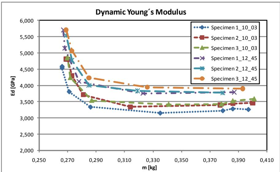
Fig. 5. The changes of Dynamic Young's modulus of chosen six specimens in dependence on weight of the specimens.
