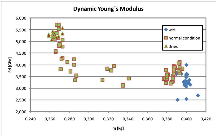
Fig. 4. The changes of Dynamic Young's modulus of all tested specimens in dependence on weight of the specimens.
