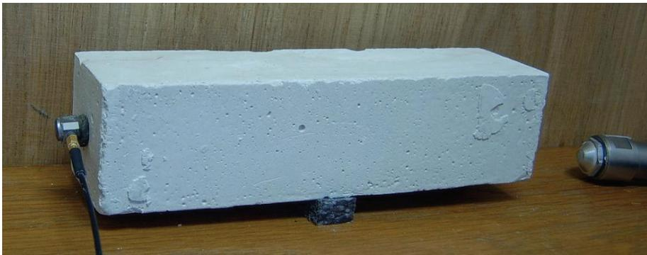
**Fig. 1.** The test arrangement for measuring the fundamental longitudinal resonant frequency of the gypsum specimen.
