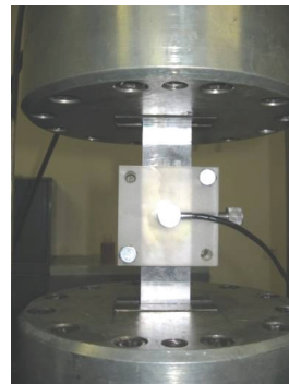
Fig. 6. Calibration sample with sensor.
