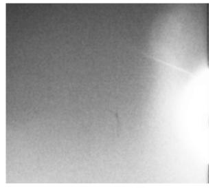
**Fig. 2.** The radiograph of elements' opening (round white area on the right side of the image) with a fatigue crack depicted as a thin bright line propagating from the opening towards upper left corner of the image.
