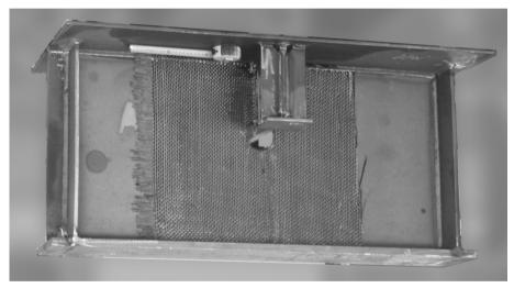
Fig. 1. Bridge element with applied carbon fibre patch on the slab with technological opening.
