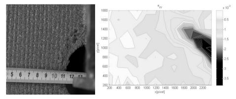
**Fig. 3.** The left part of the figure depicts two color paint sprayed on carbon fibre patch with attached measuring tape. The opening is shown as a black circular hole. On the right side of the figure strains determined by DIC method are presented in contour plots. The area of the highest strains corresponding to the darkest shadows of gray indicates the location and the extent of the crack.
