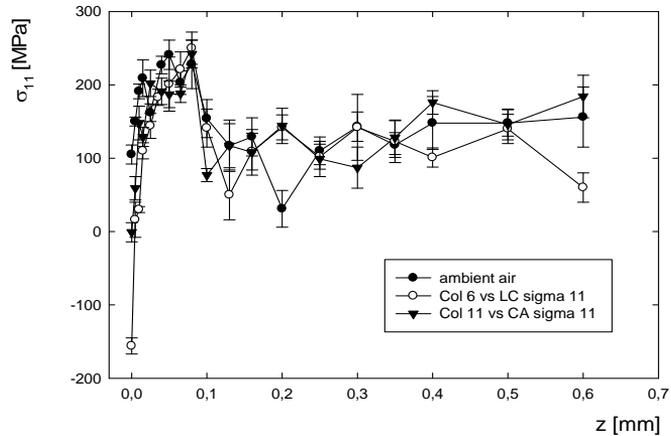
Fig. 5. Depth distribution of macroscopic residual stress  $\sigma_{11}$  in the low carbon Mn-Cr steel 16MnCr5
