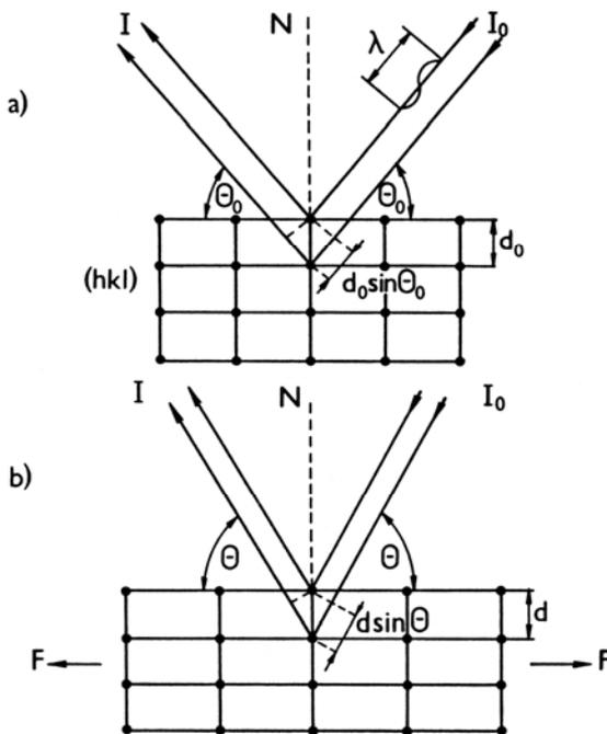
Fig. 1. Deformation of interplanar spacing and shift of the diffraction maximum.
