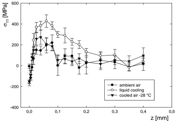
Fig. 4. Depth distribution of macroscopic residual stress  $\sigma_{11}$  in the corrosion-resistant M300 steel
