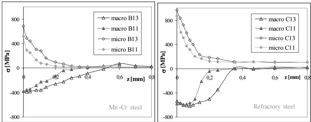
**Fig. 2.** Depth profiles of macro and micro stresses for two intensity of blasting (11-low, 13-high) for all materials *B* and *C*. The standard deviations are approximately  $\pm 30$  MPa
