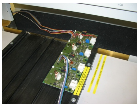
Fig. 1. Examples of PCBs with strain gauges during productions proceses
