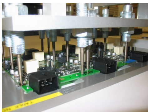
Fig. 1. Examples of PCBs with strain gauges during productions proceses
