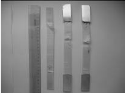
Fig. 2. Damaged specimens after static testing – set 2 (with aluminium shims)
