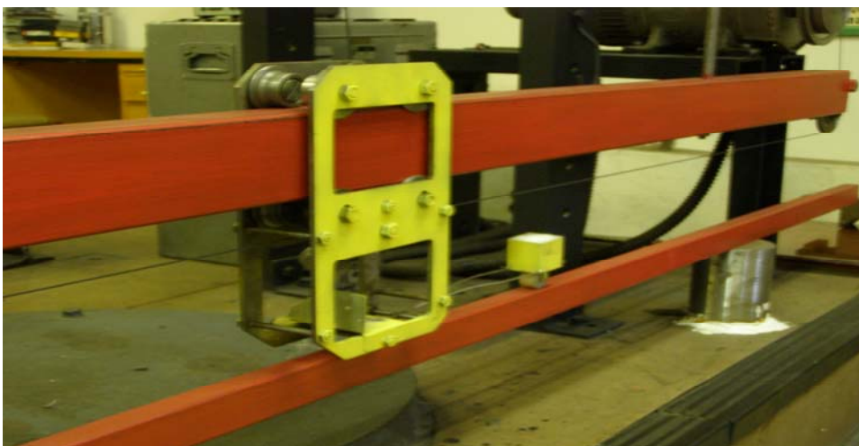
Fig. 1. Speeding-up path and equipment providing the movement of moving load
