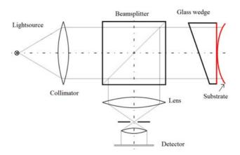
Fig. 2. Experimental setup of Fizeau interferometer
