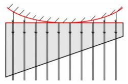
Fig. 1. Principle of Fizeau interferometry
