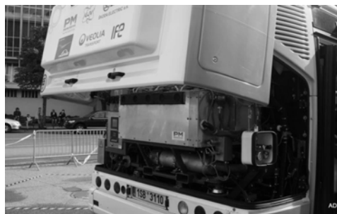
Fig. 2. Hydrogen fuel cell in the back of the TriHyBus
