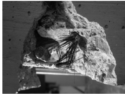
Fig. 5. Rupture of prestressed CFRP bar
