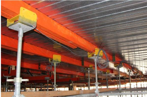
Fig. 5. Typical experimental set up with U-heads in place and cables attached.
