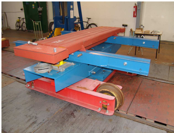
Fig. 1. Practical realization of supports - substitution test bogie
