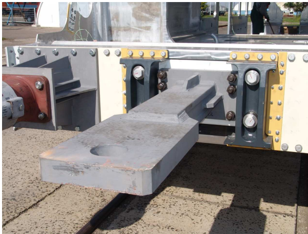
Fig. 4. Automatic coupler substitution
