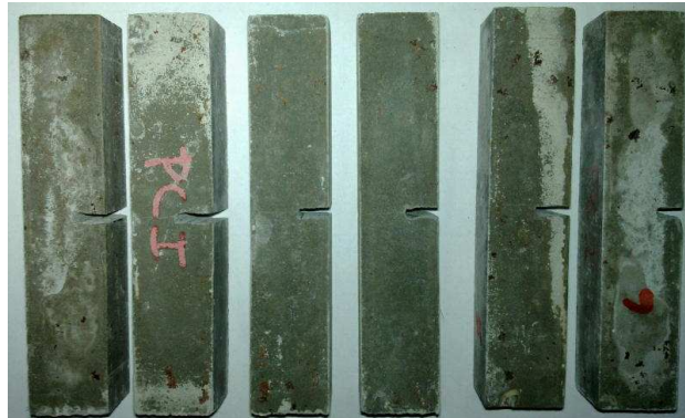
Fig. 2. Specimens after tests. Crack arises in the middle part of specimen.
