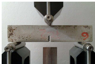
Fig. 1. Specimens with notch is prepared for three point bend test.
