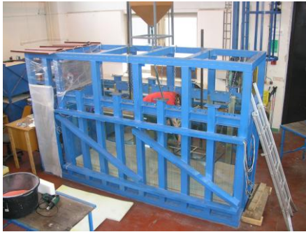
Fig. 1. Experimental equipment before the experiment E5/0,2 during sandy sample preparation.
