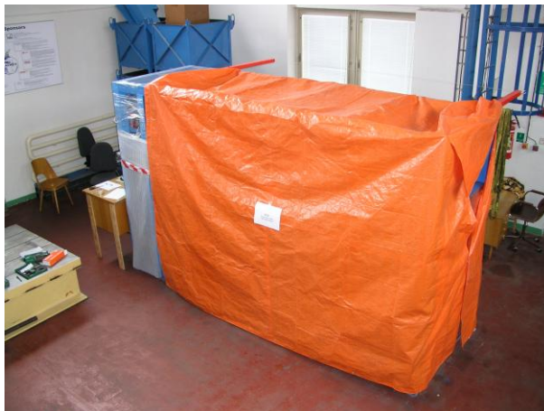
Fig. 7. Overall view at the experimental equipment under envelop against quick temperature changes whole time the experiment E5/0,2.
