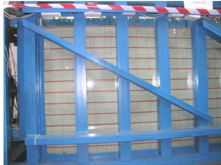
Fig. 2. Deformation of the sandy sample during the phase "recons. 4" after the toe movement of 15.6 mm (see uplift of red strips).
