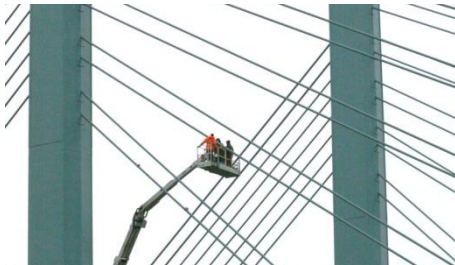
Fig. 3. Long-term cable vibration measurement
