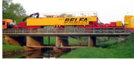
Fig. 9. Load tests using the special loading vehicle BELFA [5] www.belfa.eu
