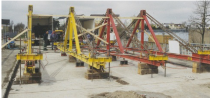
Fig. 8. Load tests using loading frameworks
