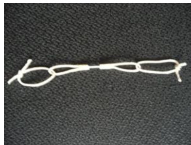
Fig. 2. Specimen for tensile test with the fixation system for avoiding off-axis load
