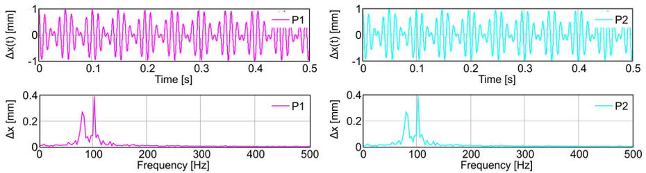
**Fig. 5.** Time and frequency dependence of oscillation displacement of cooling fan model of points P1 and P2 in x direction
