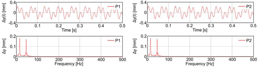
**Fig. 12.** Time and frequency dependence of automobile cooling fan vibration amplitudes in y direction determined in points P1 and P2
