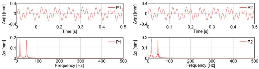
**Fig. 11.** Time and frequency dependence of automobile cooling fan vibration amplitudes in x direction determined in points P1 and P2
