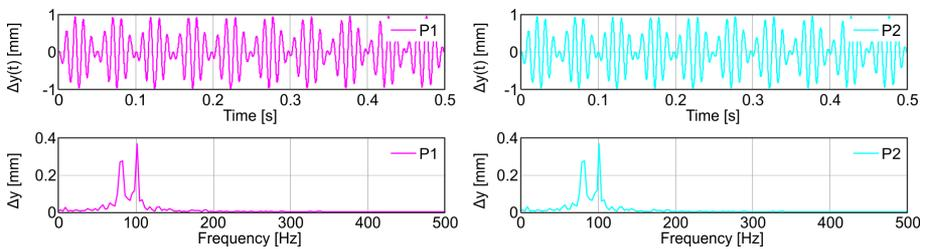
**Fig. 6.** Time and frequency dependence of oscillation displacement of cooling fan model of points P1 and P2 in y direction
