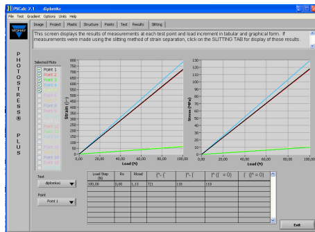
Fig. 4. Distribution of principal strains and principal normal stress displayed as a graphical output of PSCalc™ software.
