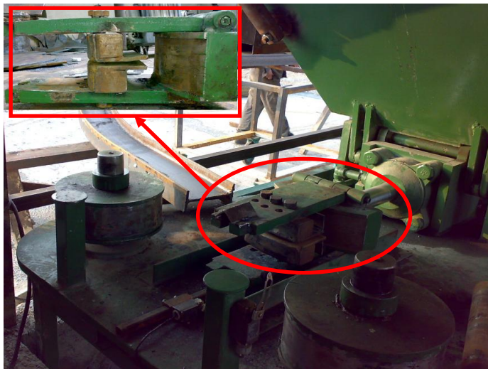
Fig. 9. Modification of the lower roller in order to prevent buckling beam web during bending
