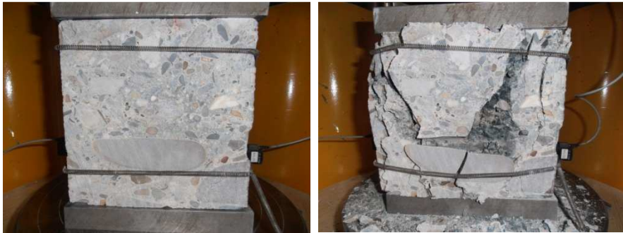
Fig. 2. Test compressive strength of concrete mixed with fly ash from Orlík dam after 50 years
