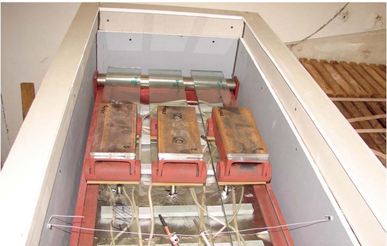
Fig. 2: Arrangement of four-point bend test in thermal chamber
